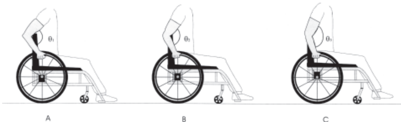
FIGURE 2: ILLUSTRATIONS A-C SHOW DIFFERENCES IN THE ELBOW FLEXION ANGLE ( Q ) FROM ADJUSTING THE HEIGHT OF THE AXLE. ILLUSTRATION B DEPICTS THE RECOMMENDED ELBOW ANGLE ( Q_2 = 100 TO 120 DEGREES). ANGLE Q_1 IS SMALLER BECAUSE THE SEAT IS TOO LOW (AXLE TOO HIGH). ANGLE Q_3 IS LARGER BECAUSE THE SEAT IS TOO HIGH (AXLE TOO LOW).
