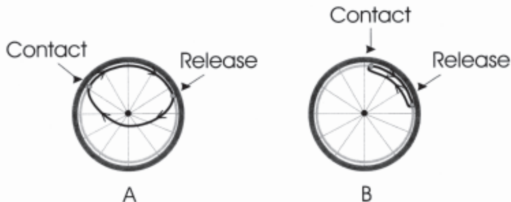
FIGURE 3: THE RECOMMENDED PROPULSION PATTERN IS SHOWN IN "A." AN EXAMPLE OF A POOR PROPULSION PATTERN IS SHOWN IN "B" (ARC PATTERN). THE THICK BLACK LINE ON THE WHEEL IS THE PATH FOLLOWED BY THE HAND.
